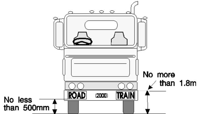
**Positioning of a warning sign****63 Left-hand drive signs**
