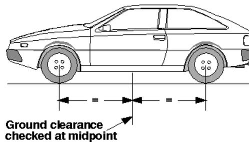
**Ground clearance at the mid-point between 2 axles**
