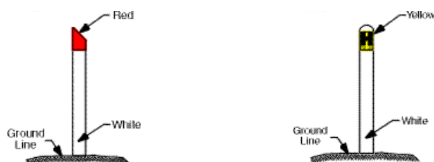
Fire hydrant indicators
