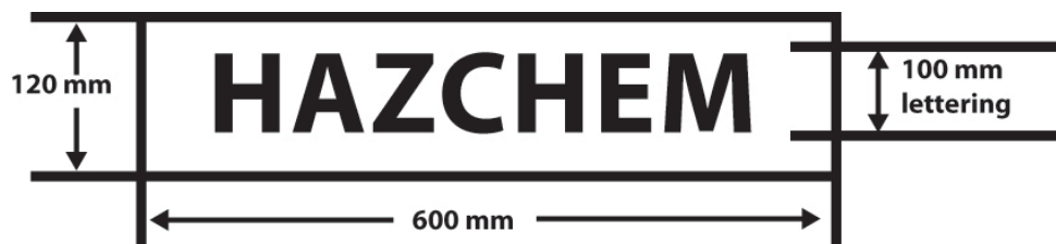
Figure 13.1 Form and dimensions of outer warning placard
