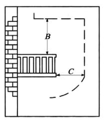
The above illustration applies if the height of the railing (or similar) PLUS distance B is greater then distance A
